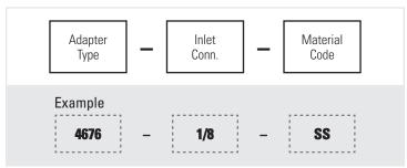
BSPT connections require the addition of a "B" in the prefix of the part number. Example: B4676.
