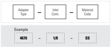
BSPT connections require the addition of a "B" in the prefix of the part number. Example: B4676.
