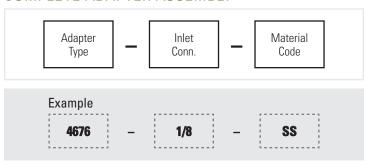
BSPT connections require the addition of a "B" in the prefix of the part number. Example: B4676.
