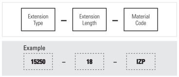
BSPT connections require the addition of a "B" in the prefix of the part number. Example: B15250.
